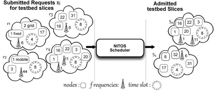
Fig. 2. Schematic diagram of the NITOS resource scheduling process.
