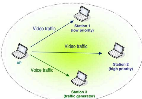
Fig. 6: The Network Setup for the Video Quality Comparison
