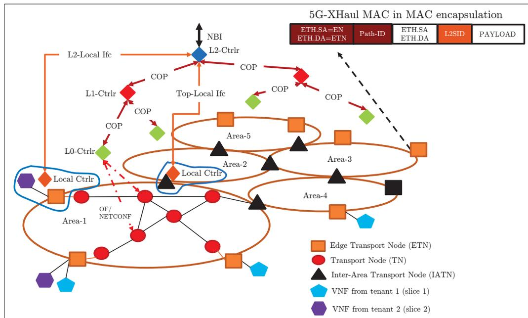
Figure 2. 5G-XHaul control plane architecture.
