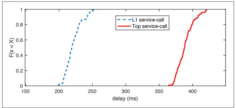
Figure 6. Control plane latency to set-up multi-domain connectivity service.
