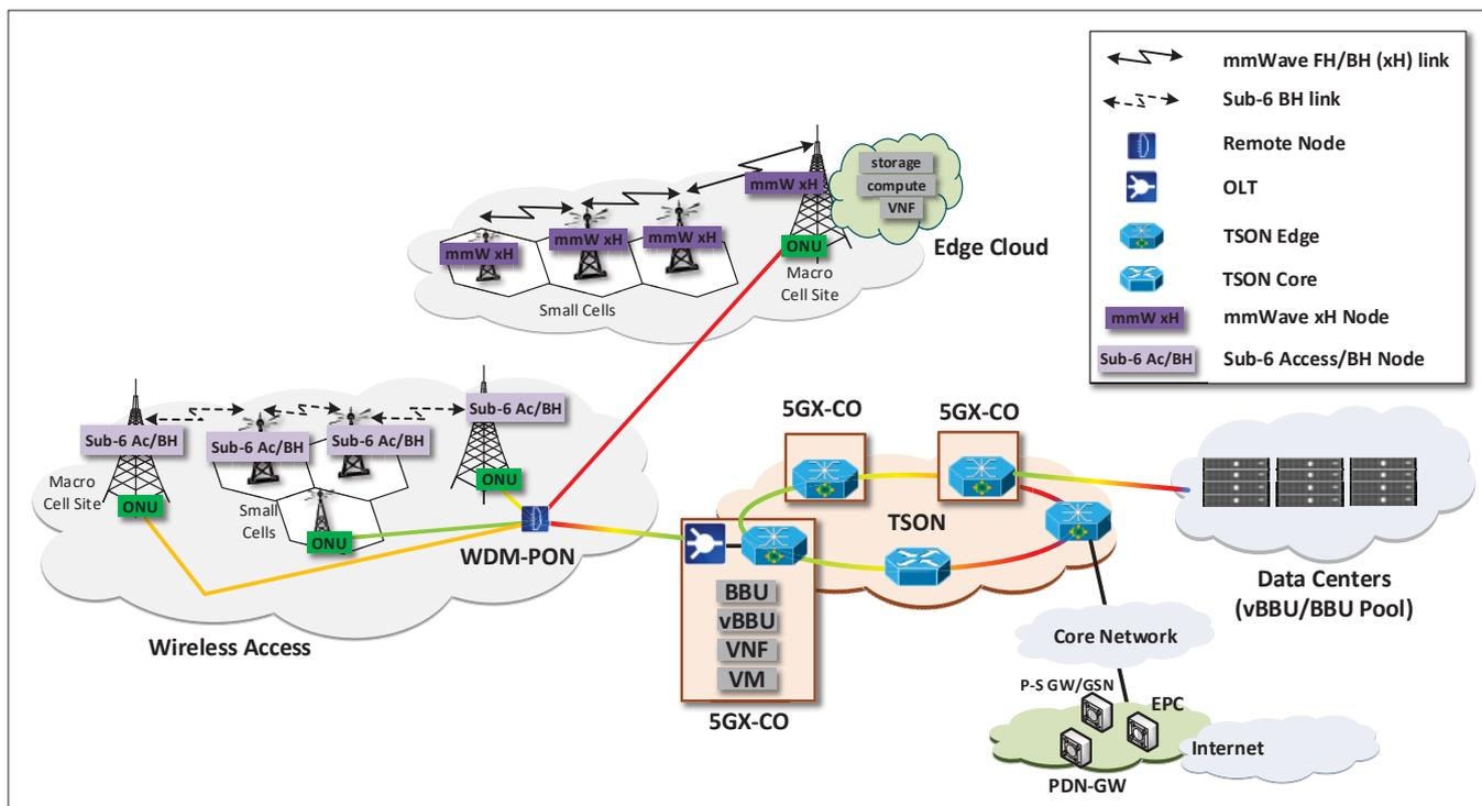
Figure 1. 5G-XHaul data plane architecture.
