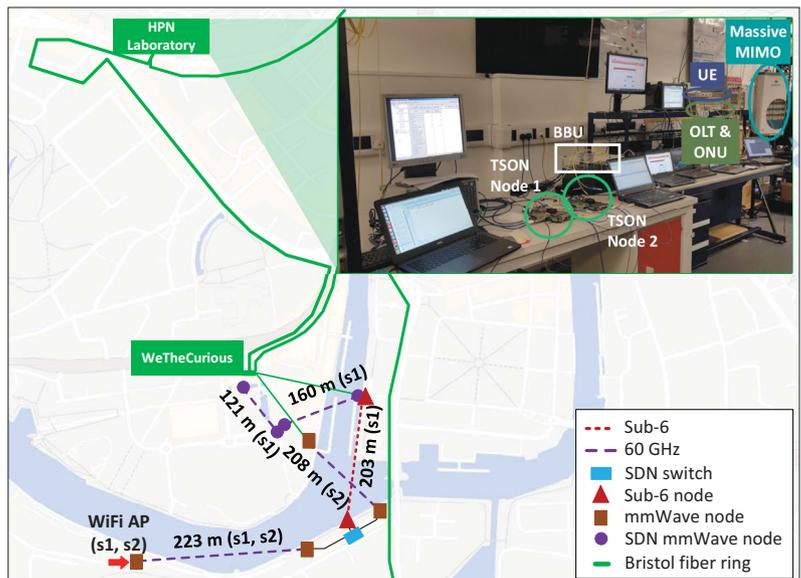
Figure 3. 5G-XHaul BiO testbed overview. Wireless SDN and optical network at HPN laboratory.
