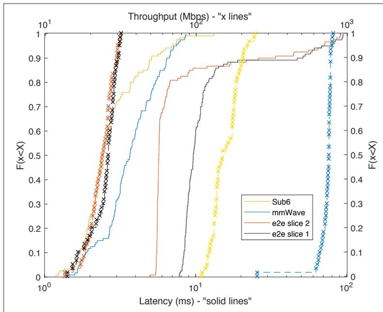
Figure 4. Benchmark of the 5G-XHaul architecture (latency/throughput).
